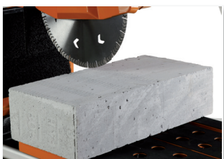
cutting depth up to 280 mm (double-sided cutting)
