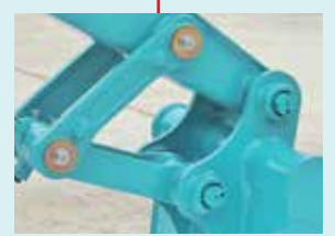
Bucket Cast-iron idler link provide greater strength.
