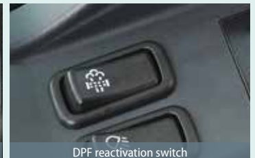
DPF reactivation switch
