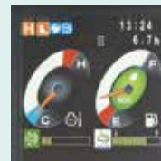
PM accumulation/ Urea accumulation display
