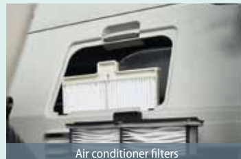
Air conditioner filters
