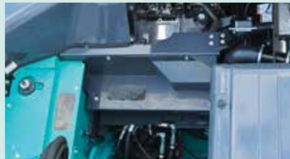
Engine maintenance Setting up maintenance area one step down allows easy to access to the engine.
