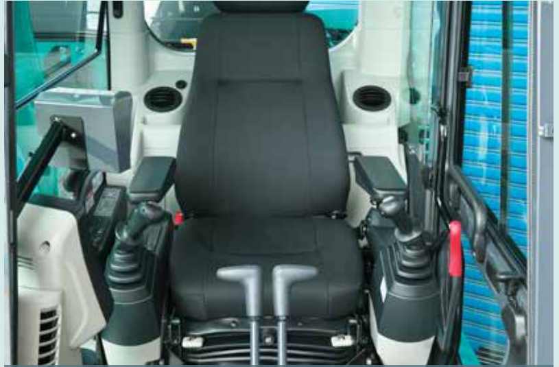
Seat suspension absorbs vibration
