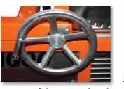
moving of the cutting head by hand wheel
