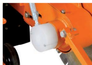
Water cooling through the blade shaft
