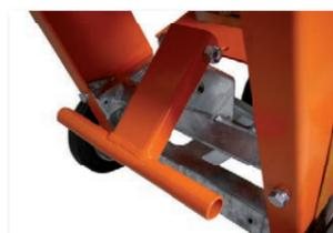
Cutting depth adjustment by foot pedal
