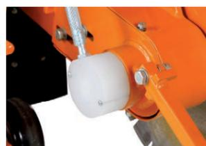
Water cooling through the blade shaft
