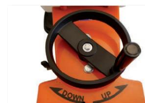
Cutting depth adjustment by handwheel
