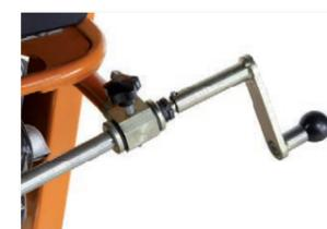
Cutting depth adjustment by handwheel
