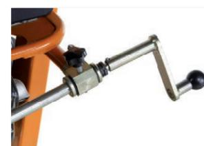
Cutting depth adjustment by handwheel
