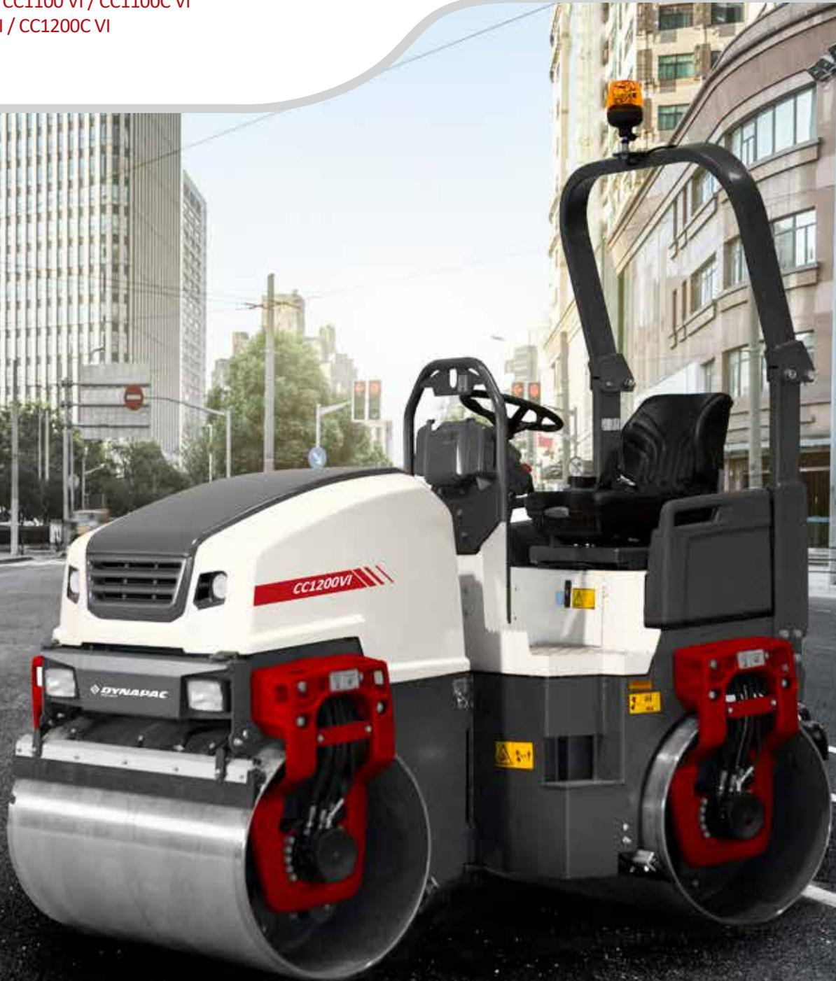
The sixth generation of the Dynapac CC1100/CC1200 VI small asphalt rollers are designed to meet the construction industry's tough conditions with the operator in mind, resulting in a robust, comfortable and modern machine for best compaction result. The new machine has a unique design with its' cross-mounted engine in combination with an excellent visibility and massive casted forks with flexible lifting/towing/tie down possibilities.
