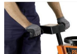
Adjustable anti vibration handles for operators comfort
