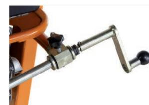
Cutting depth adjustment by handwheel
