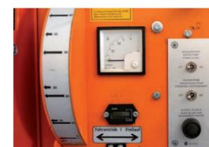
Electro-hydraulic drive, detachable. Saw can be moved without blade running.
