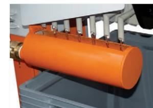
Filter outlet with drain gutter
