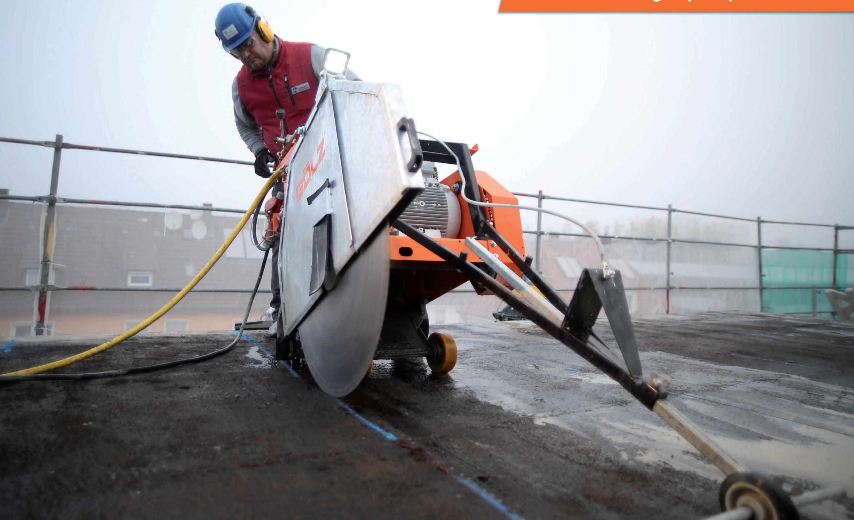
Lightweight and powerful electric floor saw, ergonomic designed for indoor applications.
