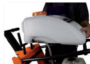
Attachable water tank 25 l, easy to fill
