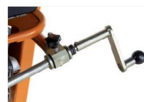
Cutting depth adjustment by handwheel
